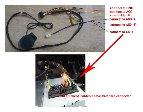
Cut off the position marked by 1 and 2.We don't need the right side part of them. Find out the B+,ACC and GND wire of original vehicle.
