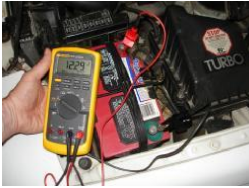
Checking base battery voltage with a voltmeter.
