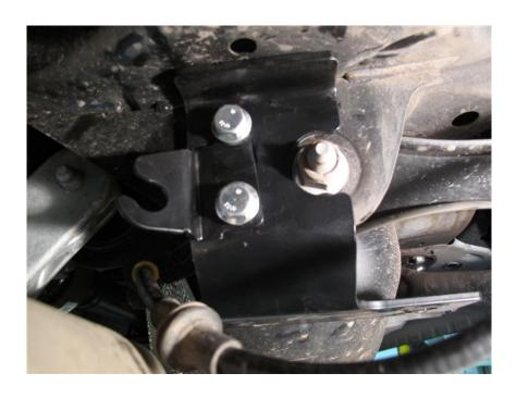
Ensure the handbrake cable is fully fitted back into the new mounting brackets,
