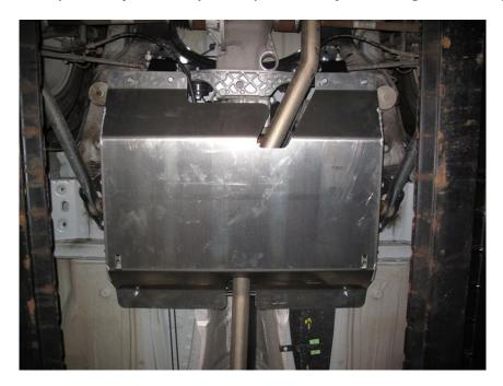
Tighten the front 2 bolts, and then lift the whole guard with either a jack or block of wood to ensure the rear mounting brackets are fully up against the vehicle structure, then tighten all the remaining rear bolts.
