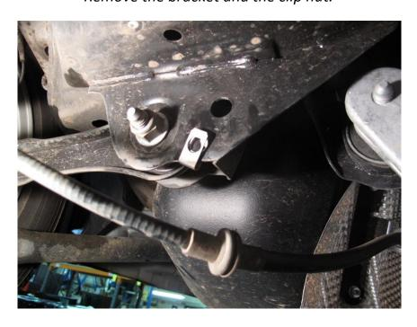
From the fitting kit, get the nut plate, left hand mounting bracket and replacement left hand handbrake cable bracket (left hand one has 3 holes in it)
