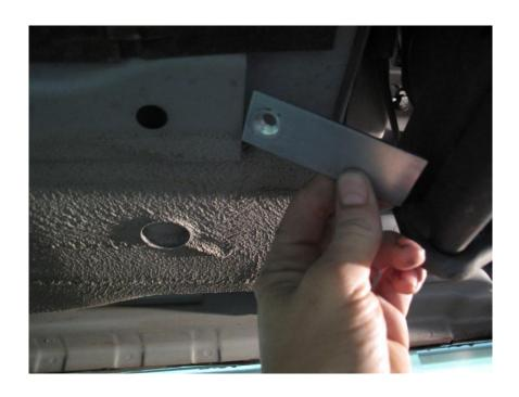
Bracket in position below, both sides of the vehicle are the same....
