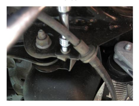
Remove the bracket and the clip nut.
