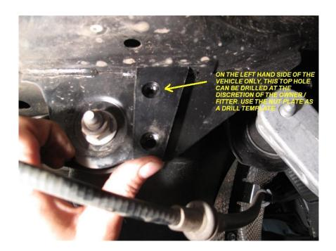
On the LEFT side of the vehicle only, the lower hole in the mounting plate is the only one which will line up, the top hole can be drilled at the fitter's choice during installation. If drilling and using 2 fixings is desired, use the nut plate as a guide to drill the top hole in the position shown above.
