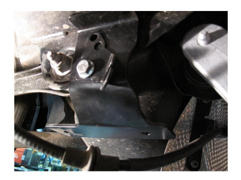
Next, repeat the same procedure on the right hand side of the vehicle using the remaining brackets in the fitting kit, loosely fit all bolts <u>DO NOT</u> tighten till instructed to do so.
