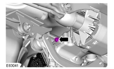
3. CAUTION: This is a filler plug only and must not be used as a fluid level indicator.
