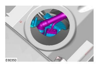
8. Disconnect the electrical connector and the breather hose.
