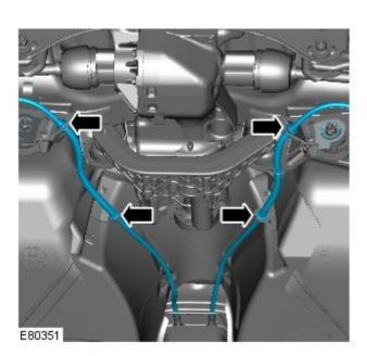
19. Release the parking brake cables from the fuel tank cradle.  $\label{eq:cables}$
