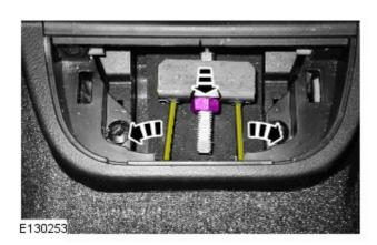
4. Release the adjusting nut and disconnect the parking brake cables from the compensator.
