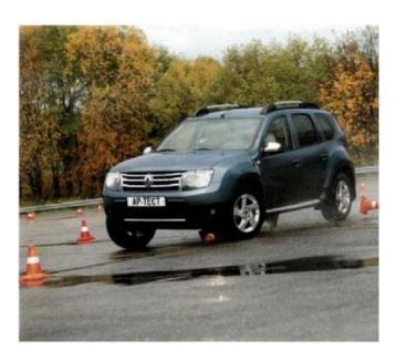
The speed was too high on entering the turn and the car skidded and knocked over a cone. But we changed the tires and the Duster easily made the turn at the same speed.
