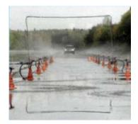
Garden sprayers helped wet the asphalt evenly for the braking distance test.
