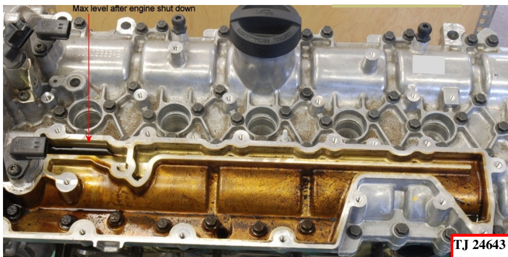
Photo 3. Oil in the breather channel indicating a possible PCV box (oil trap) failure
