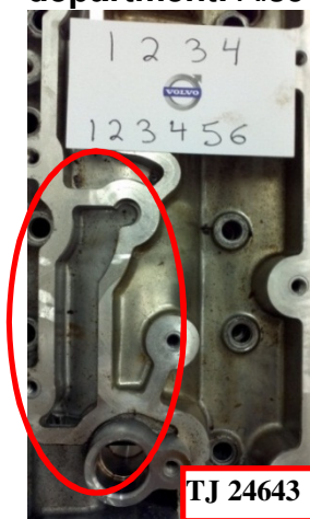
Photo 2. Intake side of PCV diaphragm
