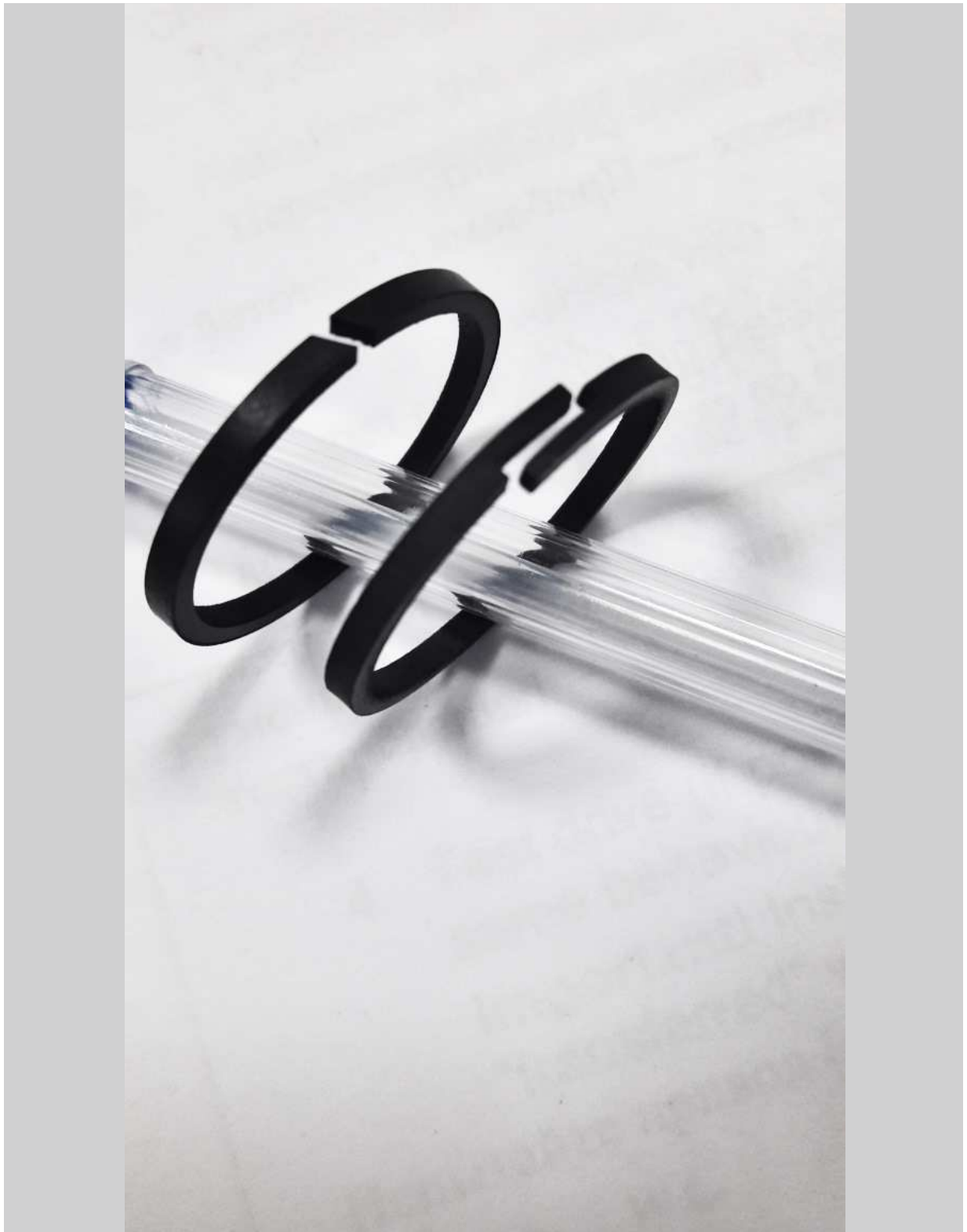
To the left is a ring of the old model, to the right - a new one, with a labyrinth seal.
