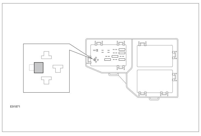
This link provides power to the entire MOST system; disruption and restoration of the power supply will initiate RBD in all nodes for up to 30 seconds after power restoration.
