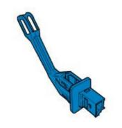
The evaporator temperature sensor is a Negative Temperature Coefficient (NTC) thermistor. The sensor is mounted on the LH side of the heater casing, and measures the temperature of cooled air once it has traveled over the evaporator. The sensor receives a 5 V reference feed from the ATC module. By monitoring the returned voltage, the ATC module can calculate the resistance of the sensor and hence evaporator temperature.
