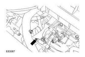
6. Loosen the bleed screw by two complete turns.
