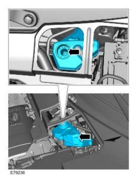
5. Attach the clear bleed tube to the clutch bleed screw and immerse the free end of the bleed tube in a bleed jar containing a small quantity of approved brake fluid.
