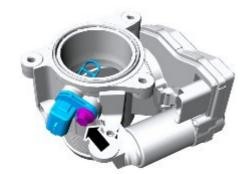
8. **8.** CAUTION: The seal is to be reused unless damaged.
