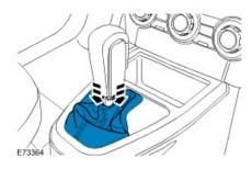
Firstly push down the gaiter just below the gear lever knob. The gear lever knob will then just pull off. The knob will pull off easily without much force.
