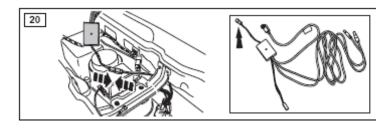
Taking the second module connect the shorter cable to the small connector from the power splitter you have just pushed under the metal cross member towards the back of the console.
