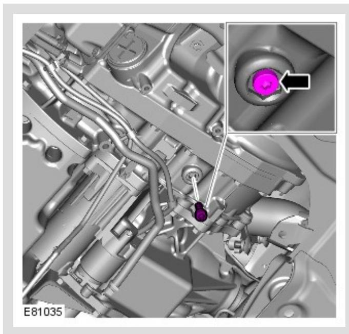
Remove the transmission fluid level plug.
