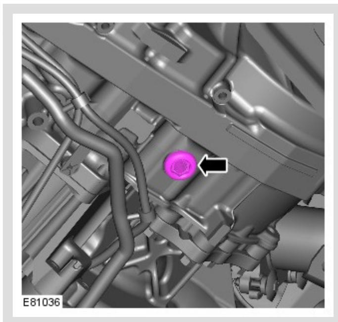
Remove the transmission fluid drain plug.
