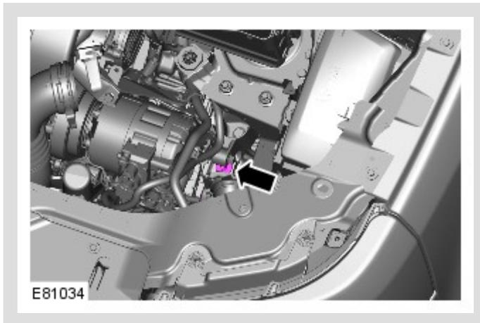
Remove the transmission fluid filler plug.
