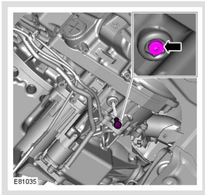
Remove the transmission fluid level plug.
