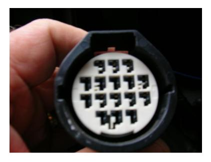
Looking at the main connector above The passenger side wire is red with a black stripe through it and the drivers side was Red with an orange stripe.. but the wires are in the same position in the plugs so just do the passenger side one then connect the drivers side to the same pin but a different colour wire.
