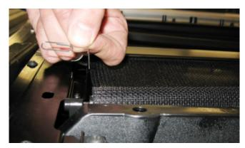
10. Assemble the rotator side of the rollo in it's mounting
