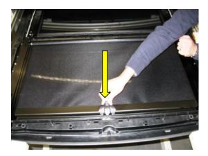
2. Rotate the rollo beam so that one of the slide shoes can taken out of the guide
