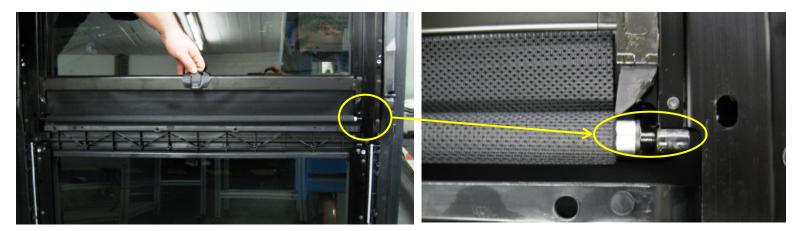
6. Now remove the other side of the rollo from it's mounting, move the rollo in direction of the arrow
