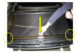
12. Rotate the rollo beam so that the other slide shoes can be inserted into the guide
