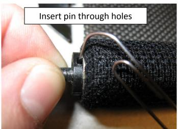
8. Assemble the spring axle into it's mounting with the pin in place to keep the tension on the rollo
