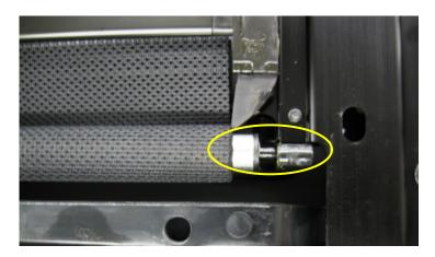
11. Move the blind to close position (do not clip to frame!) and insert one of the slide shoes into the guide
