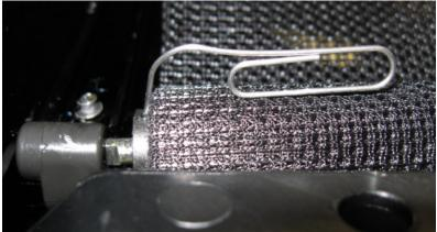
Take the pin out of the spring axle while holding the rollo tube in place (otherwise the tension is lost)
